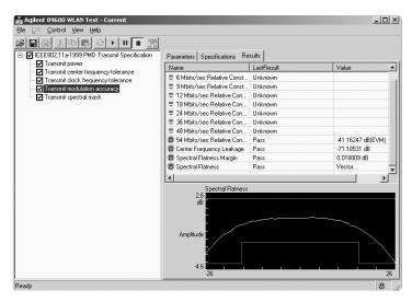
Speed standards based testing of your 802.11a/b/g WLAN transmitter with the 89607A WLAN test suite software. The test suite provides the convenience of automatic one-button test set-up and execution with the confidence of knowing your design is being tested based on the parameters and specifications set forth in the IEEE802.11a/b/g standards.
